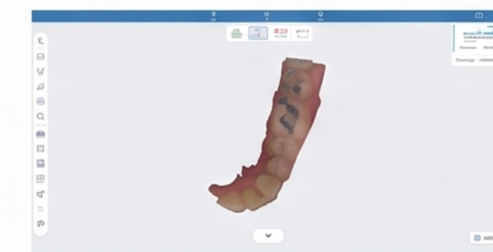
Smart Filter Automatically identifies and filters out unnecessary data such as gloves, tongue, lips, oral mucosa, and so forth
